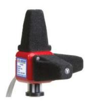
ETS-Lindgren's Model HI-6006 Electric Field Probe is a fully intelligent sensor enabling fast and accurate EMF measurements with industry-leading performance specifications. Optical coupling to a variety of readout options makes this probe ideally suited for a wide range of field monitoring applications.
